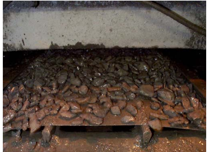
Fig. 12 Big pieces of cavings observed at the shakers due to high inclination (72°)
