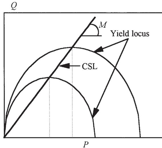
Fig. 6—Cam-Clay model, where CSL is the critical state line..
