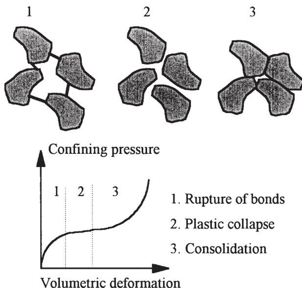
Fig. 2—Plastic collapse of a soft geomaterial.
