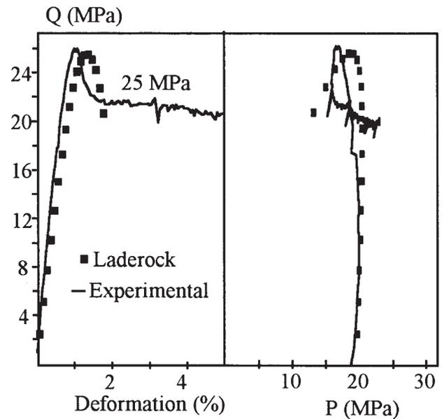
Fig. 10—Validation of Laderock on a structured clay (undrained conditions).
