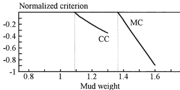
Fig. 19—Estimation of the critical instantaneous mud weight (Nuggets reservoir—vertical well), where CC is Cam-Clay and MC is Mohr-Coulomb.
