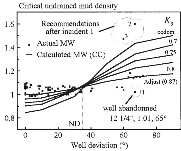
Fig. 23—Comparison of actual and calculated mud weight (MW).
