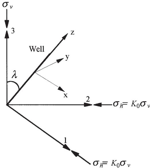
Fig. 21—Deviated well in a nonhydrostatic stress field.
