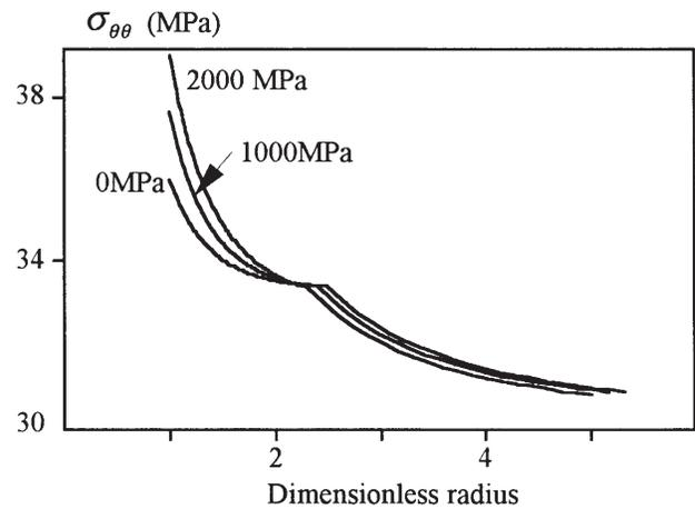
Fig. 14—Undrained pressure response in a linear strain hardening material for different values of fluid compressibility,  $k_f$ .
