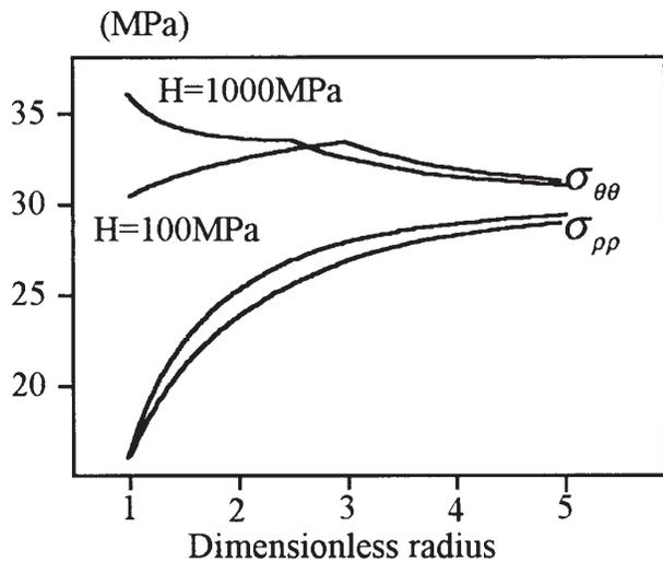
Fig. 13—Effect of strain hardening on the state of stress around a wellbore.
