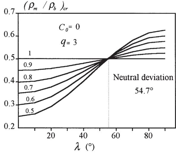
Fig. 22—Effect of  $K_0$  and deviation on critical mud weight.
