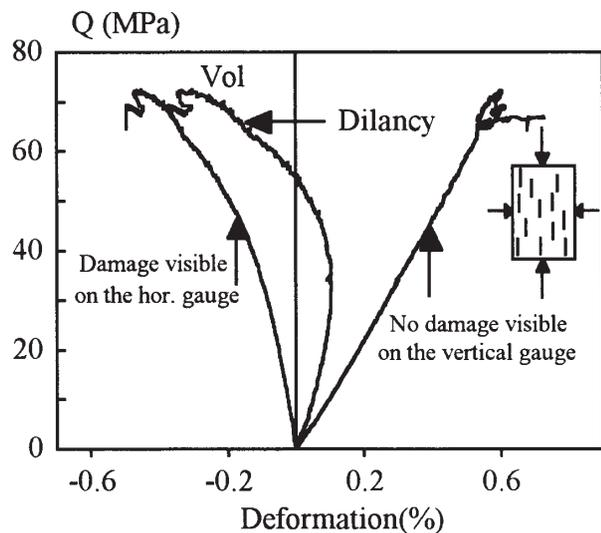
Fig. 1—Typical damaging material (Indonesian sandstone).
