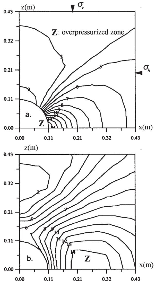
Fig. 16—Pressure distribution in a gas (a) and a water (b) saturated Cam-Clay materials.
