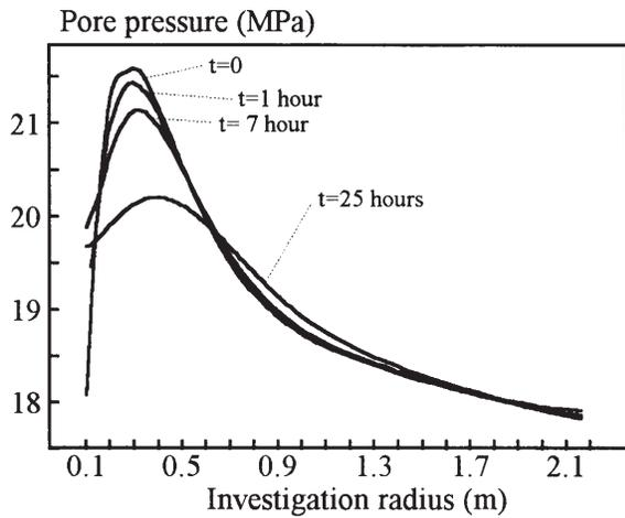
Fig. 17—Evolution of the pore pressure with time (Cam-Clay—water saturated).
