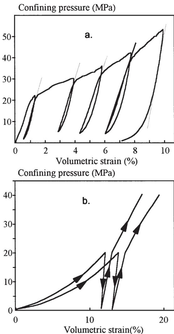
Fig. 3—Example of plastic collapse on soft porous rocks: North Sea chalk (a), Orenico sand (b).
