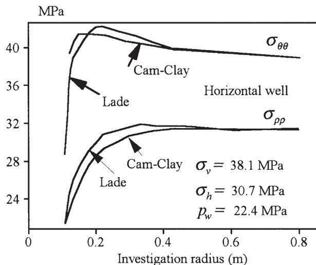
Fig. 15—Stresses obtained by Cam-Clay and Laderock models in undrained conditions (code CESAR LCPC).
