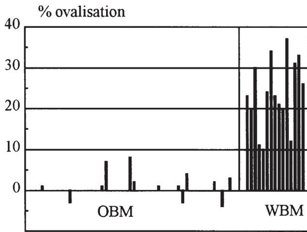
Fig. 24—Intensity of ovalization for oil-based mud (OBM) and water-based mud (WBM).
