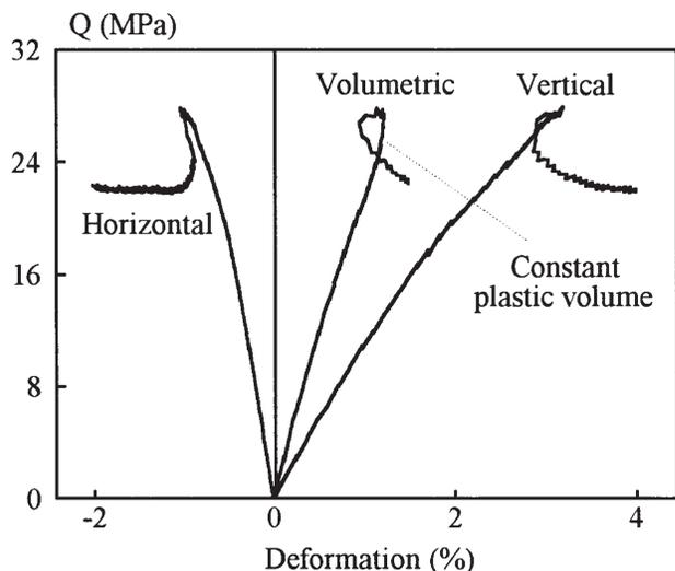
Fig. 4—Example of shear failure in a ductile rock (Villeperdue shale).
