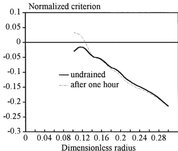
Fig. 20—Evolution of the rupture zone with time (Nuggets clay).
