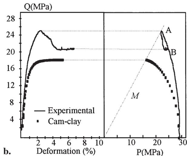
Fig. 7—Validation of the modified Cam-Clay model on an unconsolidated sand (a) and a structured clay (b).
