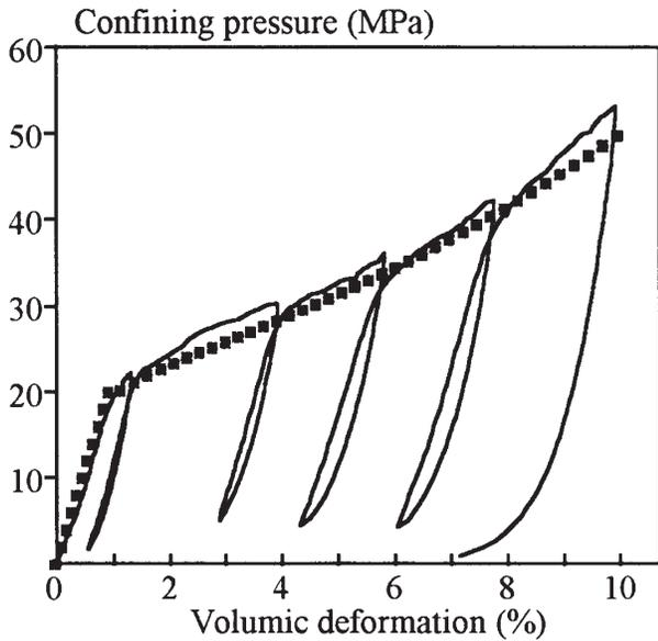
Fig. 9—Validation of Laderock on Gorm chalk (collapse mechanism only).
