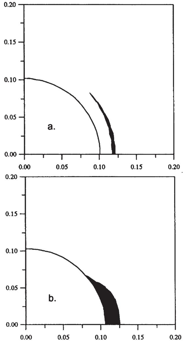
Fig. 18—Location of the rupture zone in the overburden (a) and the reservoir (b) of the Nuggets field (undrained conditions).
