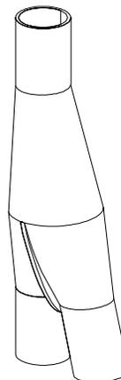
Fig. 6 Bi branch casing (developed by Marinovation)
