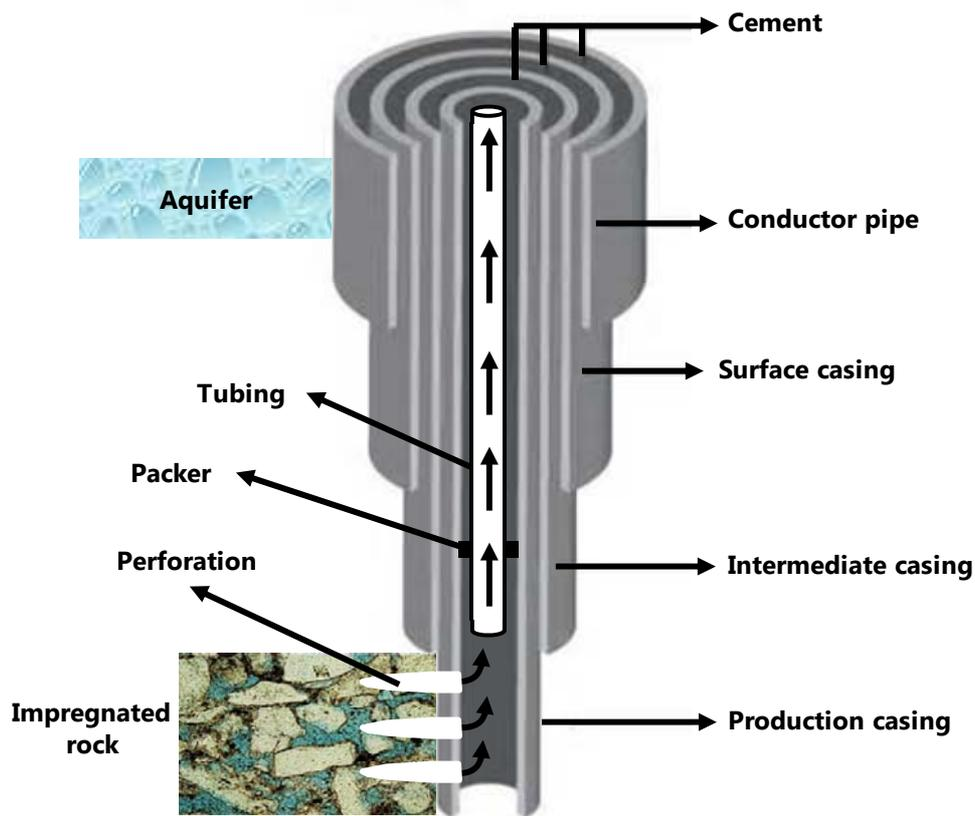
**Figure 3 – Typical well architecture.**
