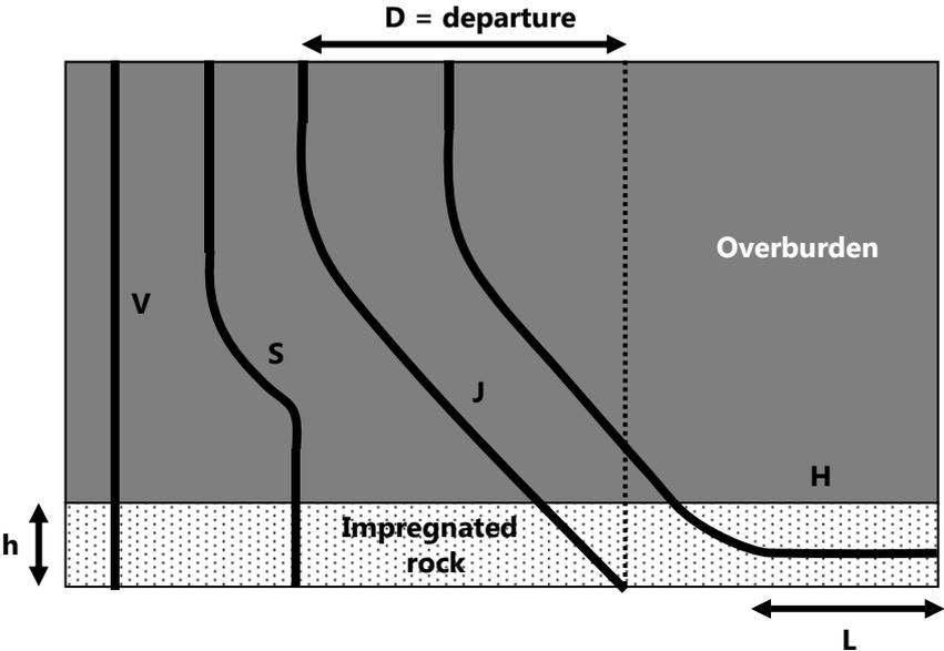
Figure 7 – Different well trajectories (V= vertical, S-shape, J=inclined, H=horizontal)
