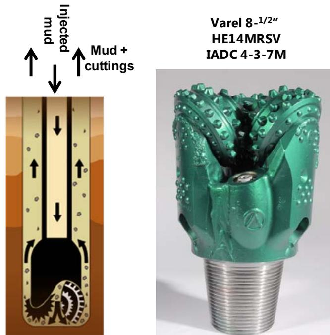
**Figure 2 – Rotary drilling and example of a drill bit (courtesy of Varel)**
