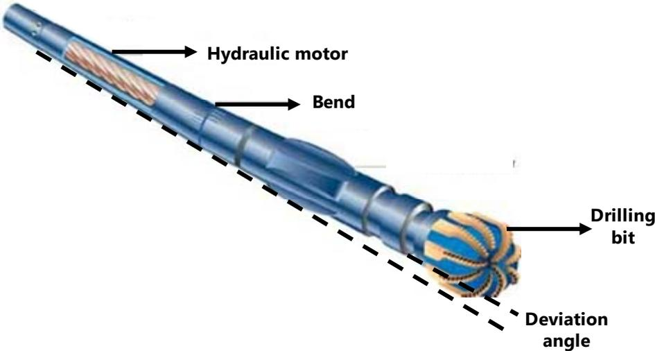
Figure 6 – Directional downhole motor
