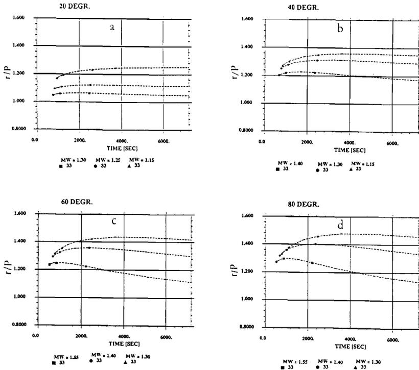
Fig. 8. Effect of consolidation on the ratio  $r/P$  for different well deviations.
