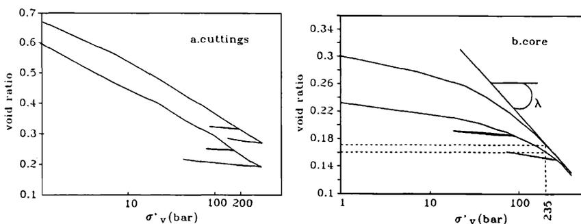
Fig. 4. Comparison of oedometric tests between cuttings and core.
