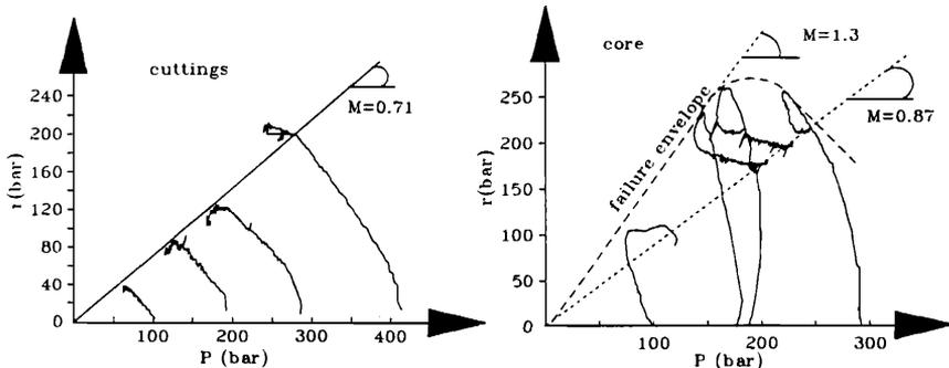
Fig. 5b. Comparison of triaxial tests between cuttings and cores
