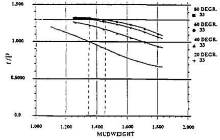
Fig.7.  $r/P$  versus mud weight for different well deviations (undrained conditions).
