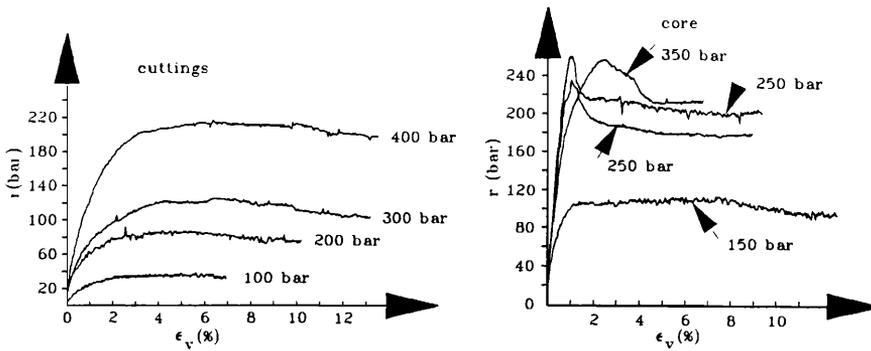
Fig. 5a. Comparison of triaxial tests between cuttings and cores
