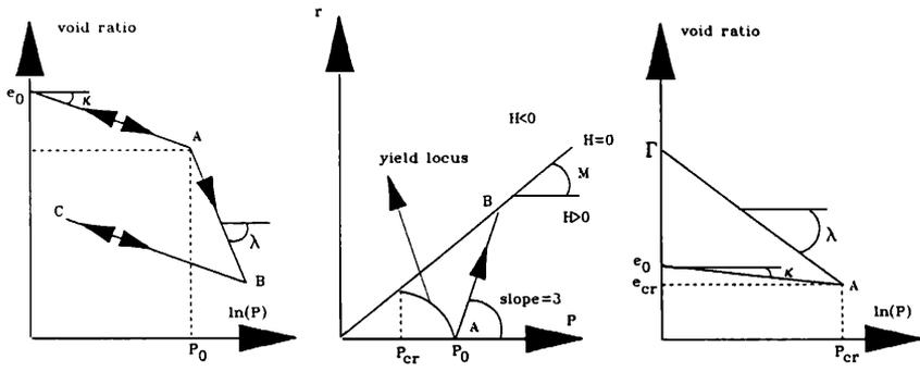
Fig. 1. Behaviour of a clay under hydrostatic compression. Fig. 2. Concept of critical state. Fig. 3. Hardening law for the Cam-Clay.
