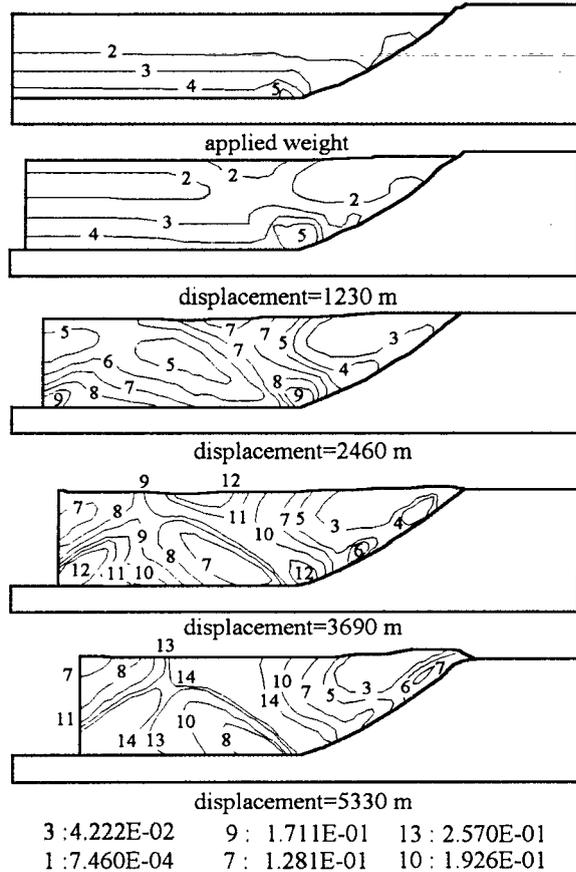
Fig 11 - Isocontours of equivalent plastic strain showing the initialization of a "pop-up".
