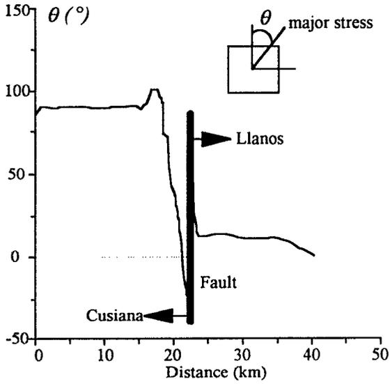
Fig. 12 Stress rotation when approaching the Cusiana fault (Mises material and zero sliding fault).
