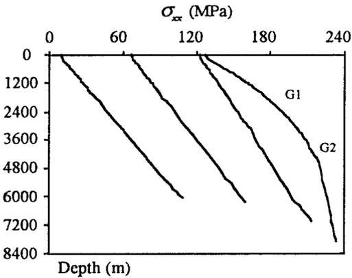
Fig. 9 - Horizontal stress profiles at different time steps
