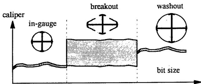
Fig. 4 - Breakout, washout and in gauge sections
