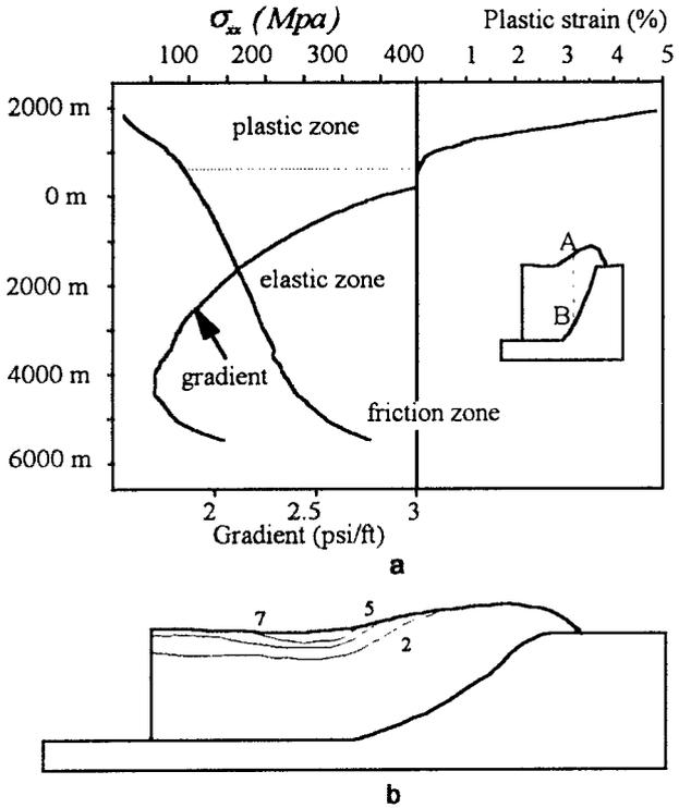
Fig. 13 - Horizontal stress profile and associated gradient for a Drucker-Prager material and a frictional fault (a) Isocontours of equivalent plastic strain (b)
