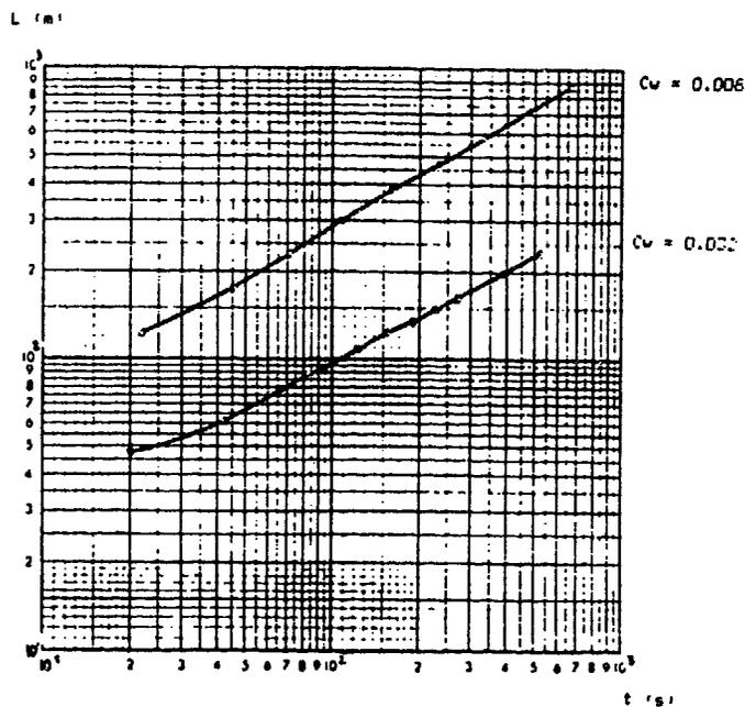
Fig. 8. Propagation restrained to E reservoir - Influence of  $C_w$  (length history)
