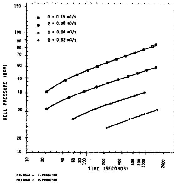
Fig. 11 Level E - Influence of flow rate on well pressure
