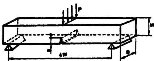
Fig. 3. Bending test to determine surface energy
