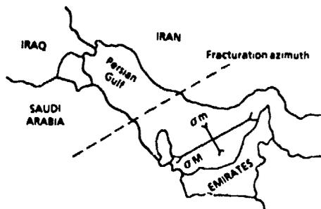
Fig. 6. Geographic orientation of the horizontal state of stress
