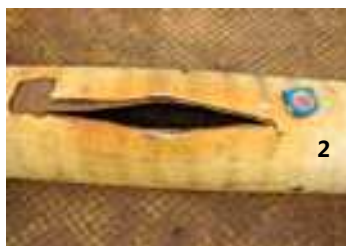
Figure 3 – Hole in a subsea oil production pipe converted into an injection pipe
