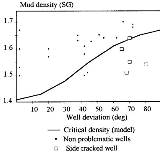
Fig 6 - Wellbore stability in Kimmeridge clay
