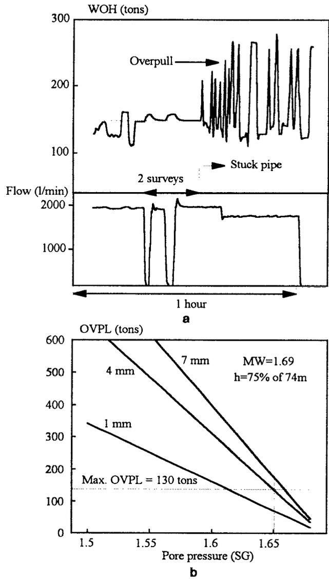
Fig. 10 Differential sticking in the Brent
