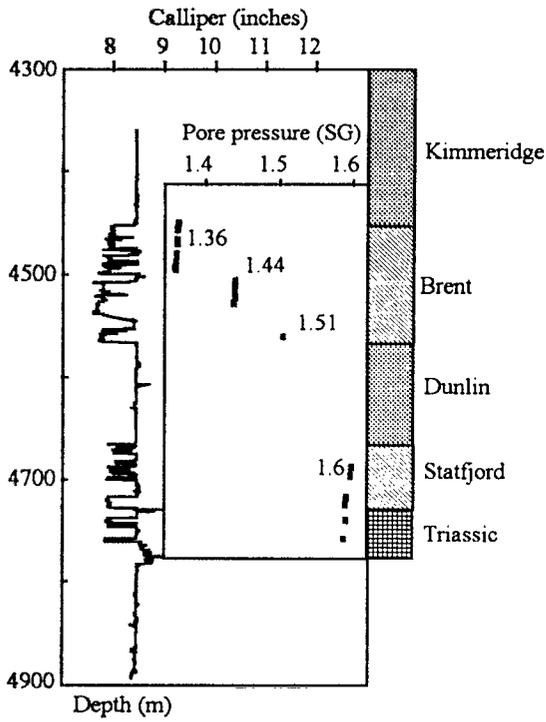
Fig 9 - Mud cake face to various depleted reservoirs
