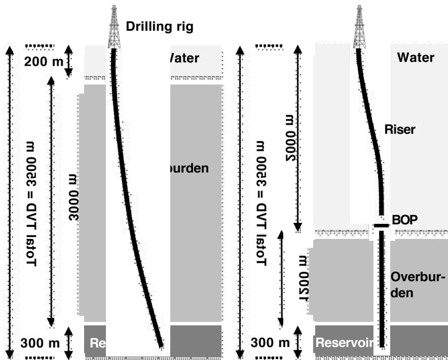
**Figure 2 – Notional comparison of a conventional offshore well and a deep offshore well**
