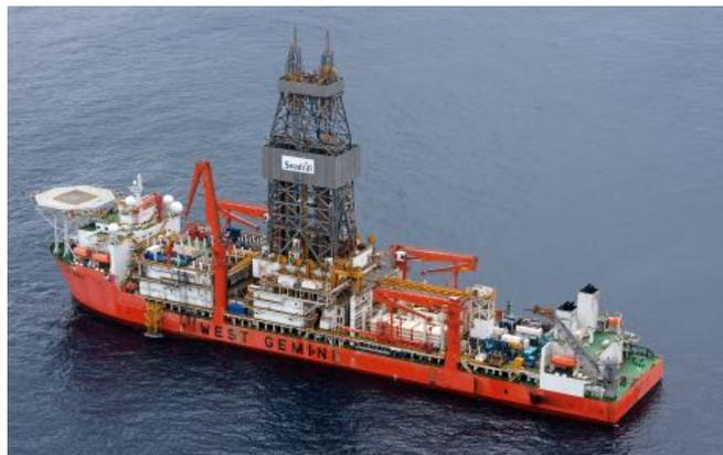
**Figure 4 – Dynamic positioning drilling rig**
