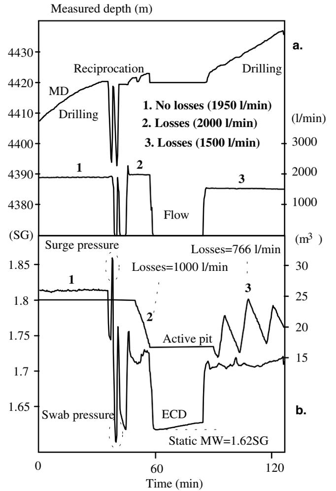
**Fig. 7 Losses in an induced fracture following a surge peak**
