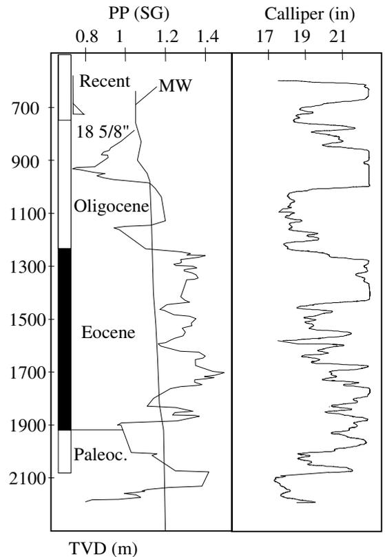
Fig. 4 Example of highly unstable shales when drilled in underbalanced conditions
