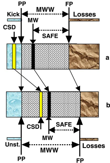
Fig. 3 Comparison of MWW in a passive basin
