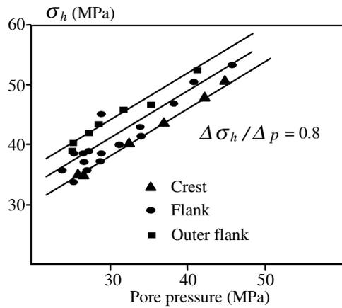
**Fig. 10 - Strong dependence between pore pressure and minimal stress on the Ekofisk field (according to Teufel and al, 1991)**
