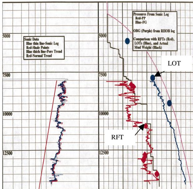
Fig. 2 Example of MWW issued from the software Drillworks/PREDICT
