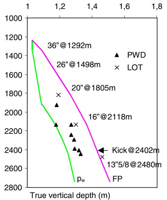
**Fig. 18 Example of MWW of a deep water Well in the Gulf of Mexico**
