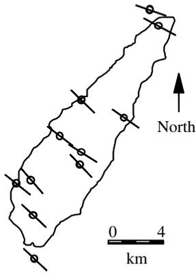
**Fig. 14 Well ovalisation and direction of tectonic thrust in the Cusiana field**
