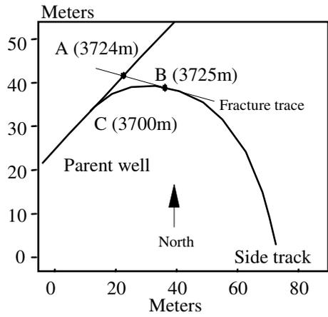
**Fig. 9 - Losses in a natural fracture crossing both the parent hole and the re-entry.**
