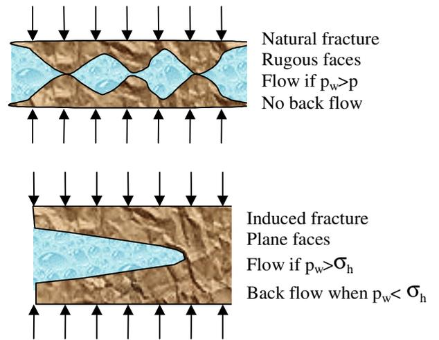
**Fig. 8 - Comparaisn between a natural (a) and an induced fracture (b)**
