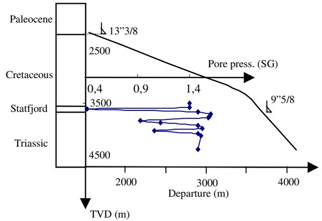
**Fig. 12 Special casing design and trajectory when coupling depleted and undepleted reservoirs (Alwyn field - North Sea)**
