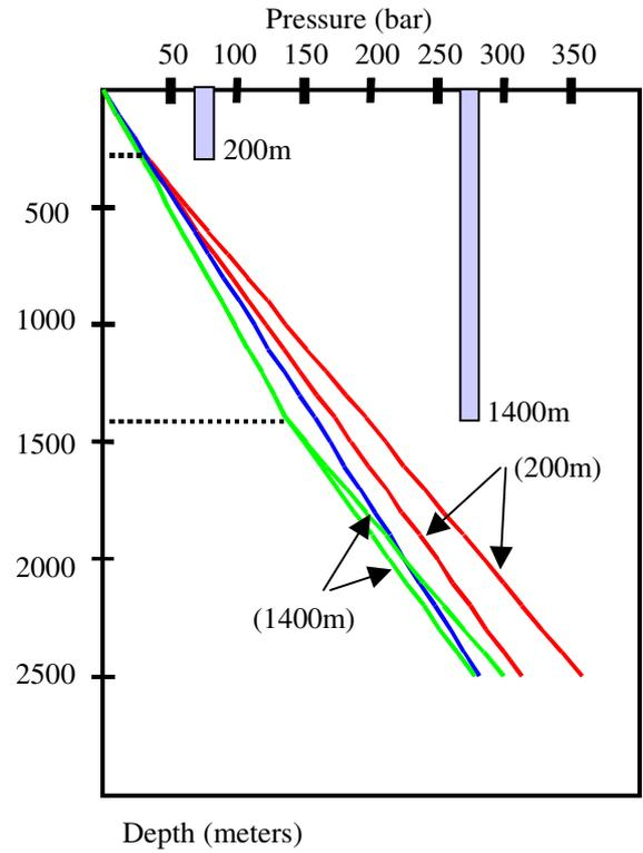
**Fig. 17 Mud weight window in the case of a deep water well**
