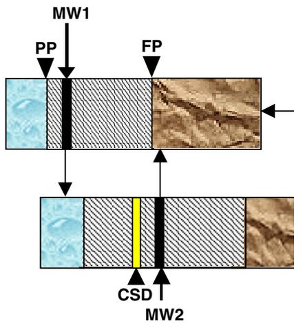
**Fig. 11 Incompatibility between an unstable shale and a depleted reservoir.**
