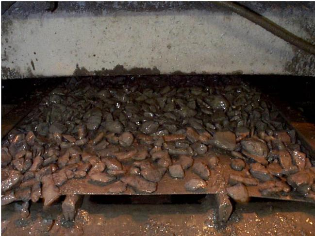
**Fig. 5 Large amounts of cavings following underbalanced conditions in highly unstable shales**
