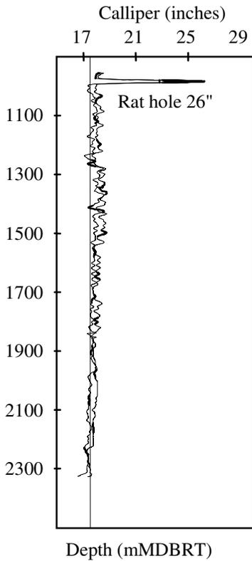
**Fig. 6 - In-gauge well according to the new overbalanced mud weight strategy.**
