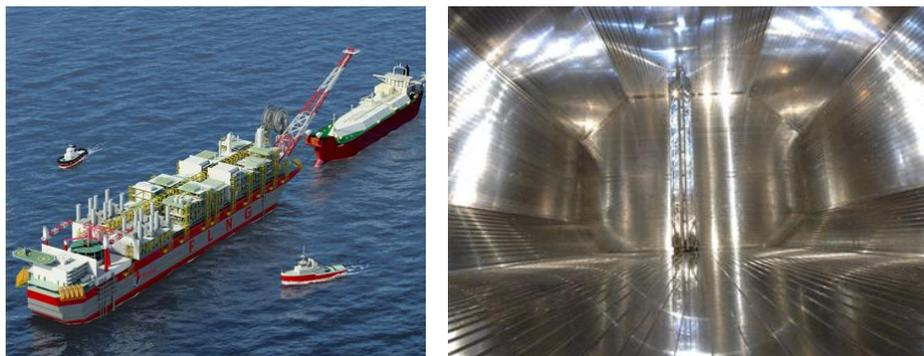
**Figure 2 – Synthetic view of what could be a FLNG unit with tandem offloading. LNG storage chamber.**
