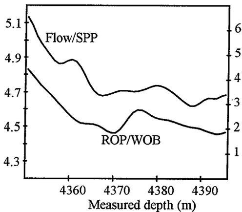
Fig. 9 Plugging of the downhole motor at the end of the third run.
