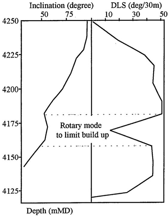
Fig. 5 Inclination and DLS of the kick-off section
