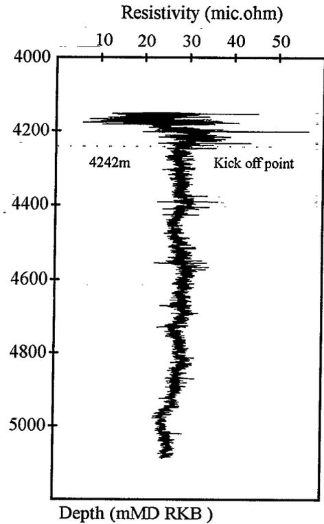
Fig.11 Resistivity log along the lateral drain.
