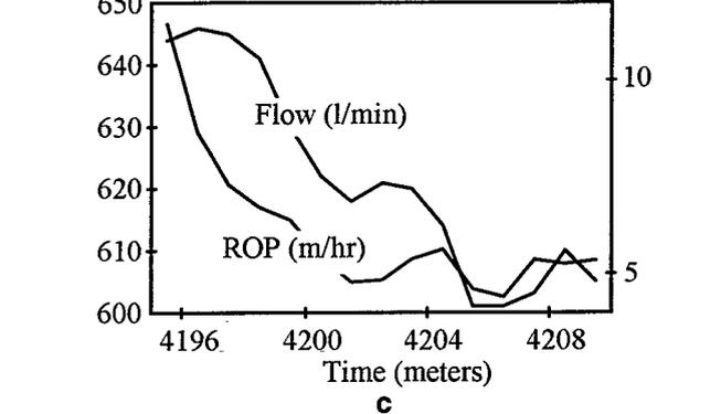
Fig. 7 Losses at 3725m TVD
