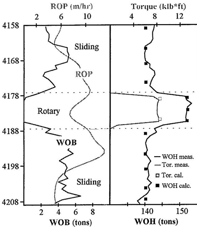
Fig. 6 Kick-off section Drilling parameters during the first section
