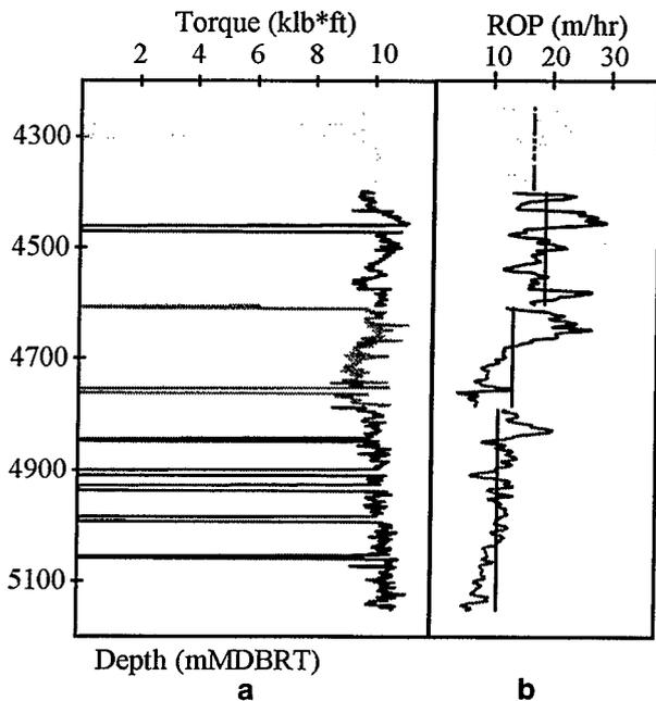
Fig. 10 a. Surface torque (drops correspond to sliding mode)
